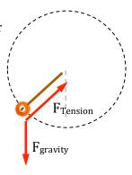
With these axes in mind, we can see that we'll have to split the force of gravity up into components, and then use  $F_{net} = ma$  to calculate the force of tension.
