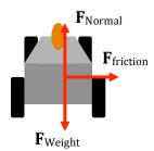
b. For the car to be able to make it around the turn, it needs a centripetal force of
