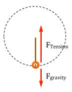
This is much greater than the weight of the billiard ball by itself, just 1.47 N. That's because the Tension in the string has to support the weight of the ball, *and* accelerate the ball toward the middle of the circle so that it will travel in that circular path.
