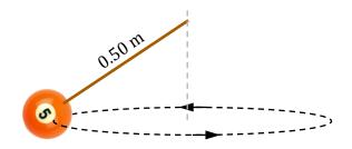
c. Determine the magnitude of the centripetal acceleration of the ball as it travels in the horizontal circle.
