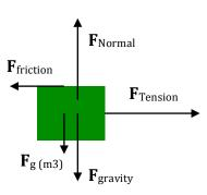
opposite the force of Tension, and keeps  $m_2$  from accelerating as quickly as it would otherwise.
